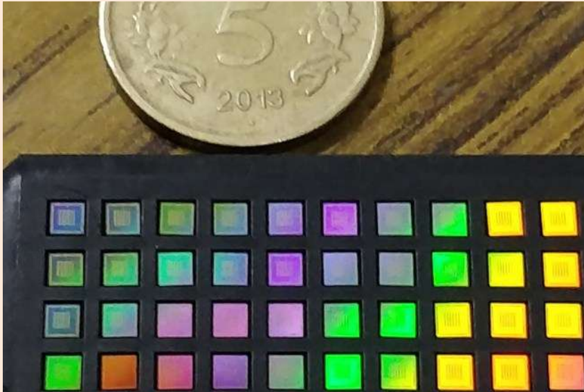
Small silicon dies with exploratory neuromorphic devices and circuits designed at Suri lab at IIT-Delhi
